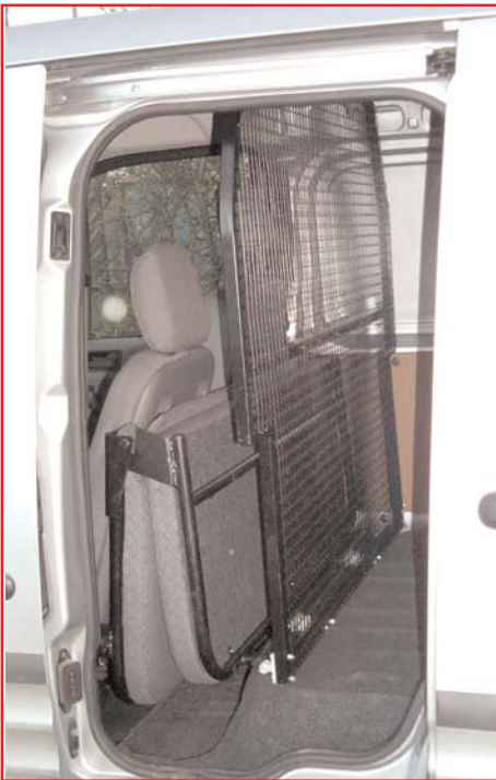
Example of seat folded up with mesh bulkhead in Ford Connect moved forward still leaving 85% of the vans carrying capacity
